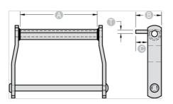
NOTE: All dimensions shown in inches unless noted otherwise. C1/2 attachment is welded to front of barrel.
