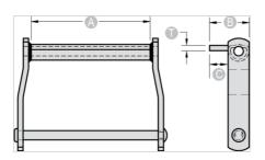
NOTE: All dimensions shown in inches unless noted otherwise. C1 attachment is welded on top of barrel.
