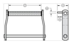
NOTE: All dimensions shown in inches unless noted otherwise. C4 attachment is welded on top of barrel.
