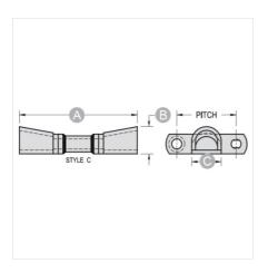
NOTE: All dimensions shown in inches unless noted otherwise. A and B dimensions can easily be altered to meet requirements. Specify A and B dimensions when inquiring.
